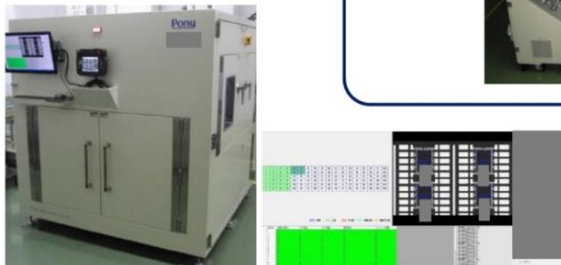
Mold後全数X-Ray検査
