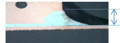
Wettable flank 0.14mm
